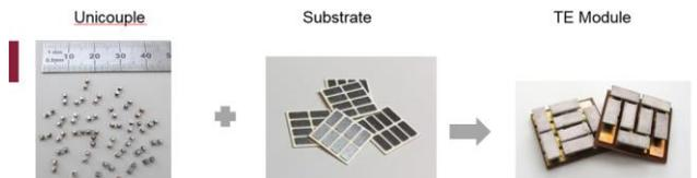
Fig. 2. Two step manufacturing of a thermoelectric module
